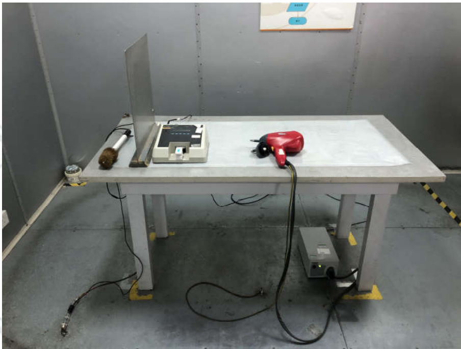
Electrostatic Discharge Test Setup
