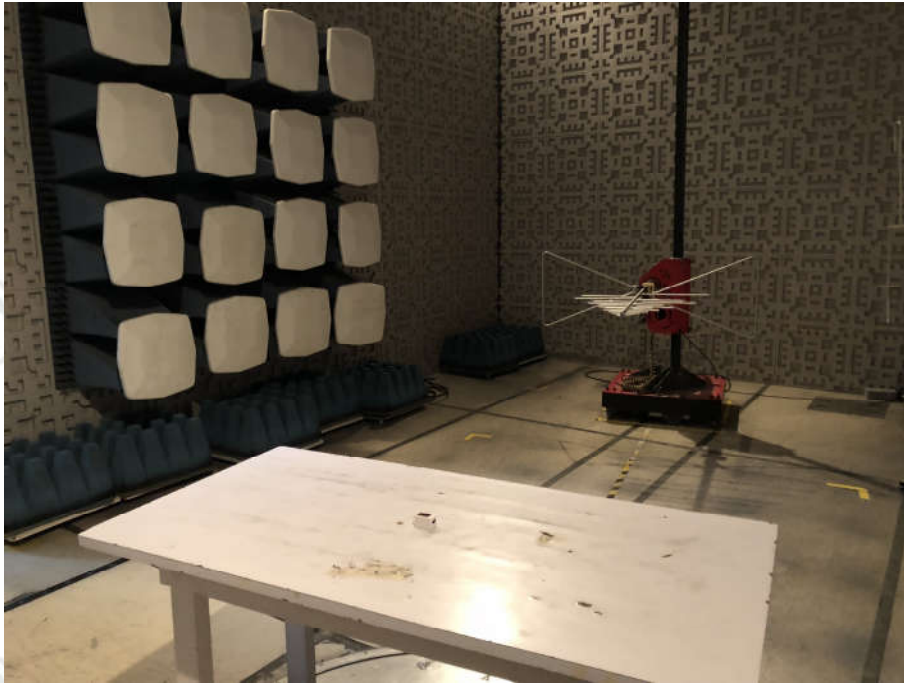
Radiation Disturbance Test Setup
